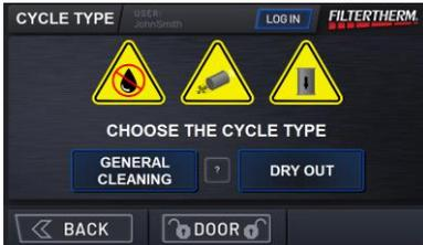
The GENERAL CLEANING CYCLE will heat to the temperature requirements set by the DPF manufactures.
